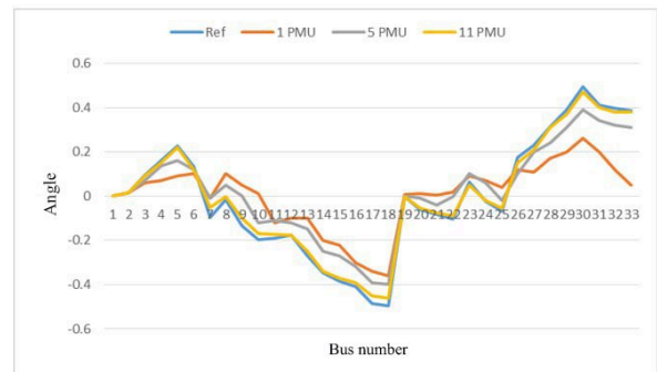
Figure 5: The impact of different numbers of PMUs on voltage angle value
